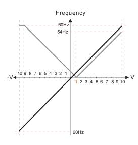
Pr.00-21=0 (Dgital keypad control and d run in FWD direction) Pr.03-05 Analog Positive Voltage Input Bias (AUI) = 10%
