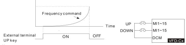
Pr.02-09 set to 1: it will increase/decrease frequency command (F) by the setting of acceleration/deceleration (Pr.01-12~01-19) and only be valid during operation.
