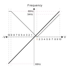
Pr.00-21=0 (Dgital keypad control and d run in FWD direction)
