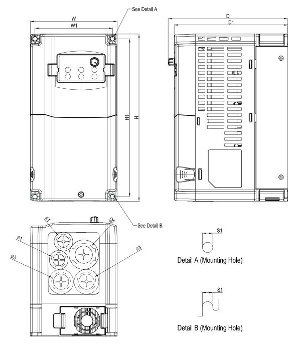
Unit: mm [inch] W1 W Н D H1 D1 S1 Ф1 Ф2 Ф3 130.0 250.0 179.0 116.0 236.0 170.0 6.2 22.2 34.0 28.0 [5.12] [9.84] [7.05][4.57] [9.29] [6.69][0.24][0.87][1.34] [1.10]
