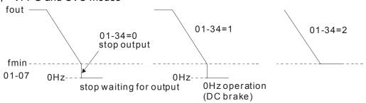
In FOCPG mode, when Pr.01-34 is set to 2, it will act according Pr.01-34 setting.
