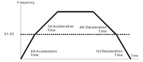
1st/4th Acceleration/Deceleration Frequency Switching
