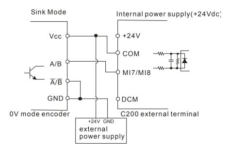
5. Since MI1~MI8 shares the same COM, therefore when using a PG card, MI~MI6 can only be applied at SINK MODE.
