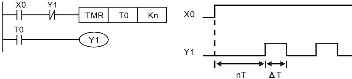
The figure above uses timer T0 to control coil Y1 to be ON. After Y1 is ON, timer T0 will be closed at the next scan period and output Y1. The oscillating circuit will be shown as above. (n is the setting of timer and it is decimal number. T is the base of timer. (clock period))
