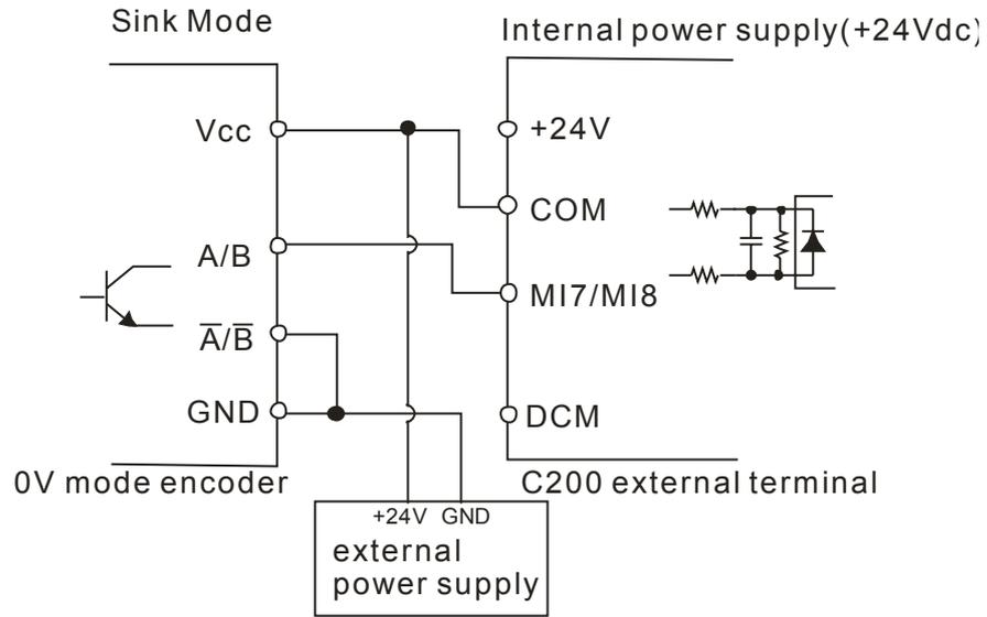
5. Since MI1~MI8 shares the same COM, therefore when using a PG card, MI~MI6 can only be applied at SINK MODE.
