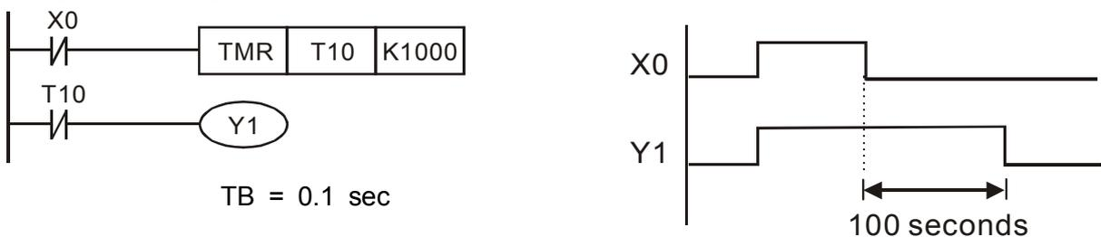
When input X0 is ON, output coil Y1 will be ON at the same time due to the corresponding normally close contact OFF makes timer T10 to be OFF. Output coil Y1 will be OFF after delaying 100 seconds ( $K1000 \cdot 0.1 \text{ seconds} = 100 \text{ seconds}$ ) once input X0 is OFF and T10 is ON. Please refer to timing chart above.
