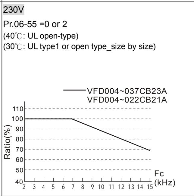
**Derating curve diagram in the normal duty (Pr.00-16=0)**
