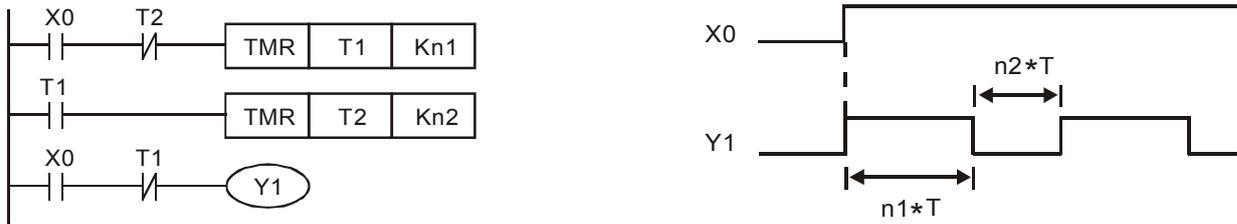
The figure above is common used oscillating circuit for indication light blinks or buzzer alarms. It uses two timers to control On/OFF time of Y1 coil. If figure, n1 and n2 are timer setting of T1 and T2. T is the base of timer (clock period)
