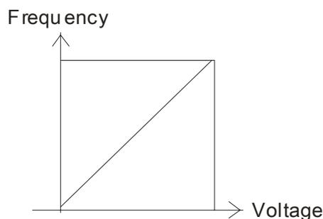
$$F_{\text{command}} = [(a_y - \text{bias}) * \text{gain}] * \frac{F_{\text{max}}(01-00)}{10\text{V or }16\text{mA}}$$
