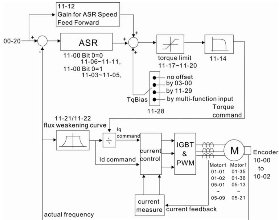
When setting Pr.00-11 to 6, PM FOC sensorless control diagram is shown as follows:
