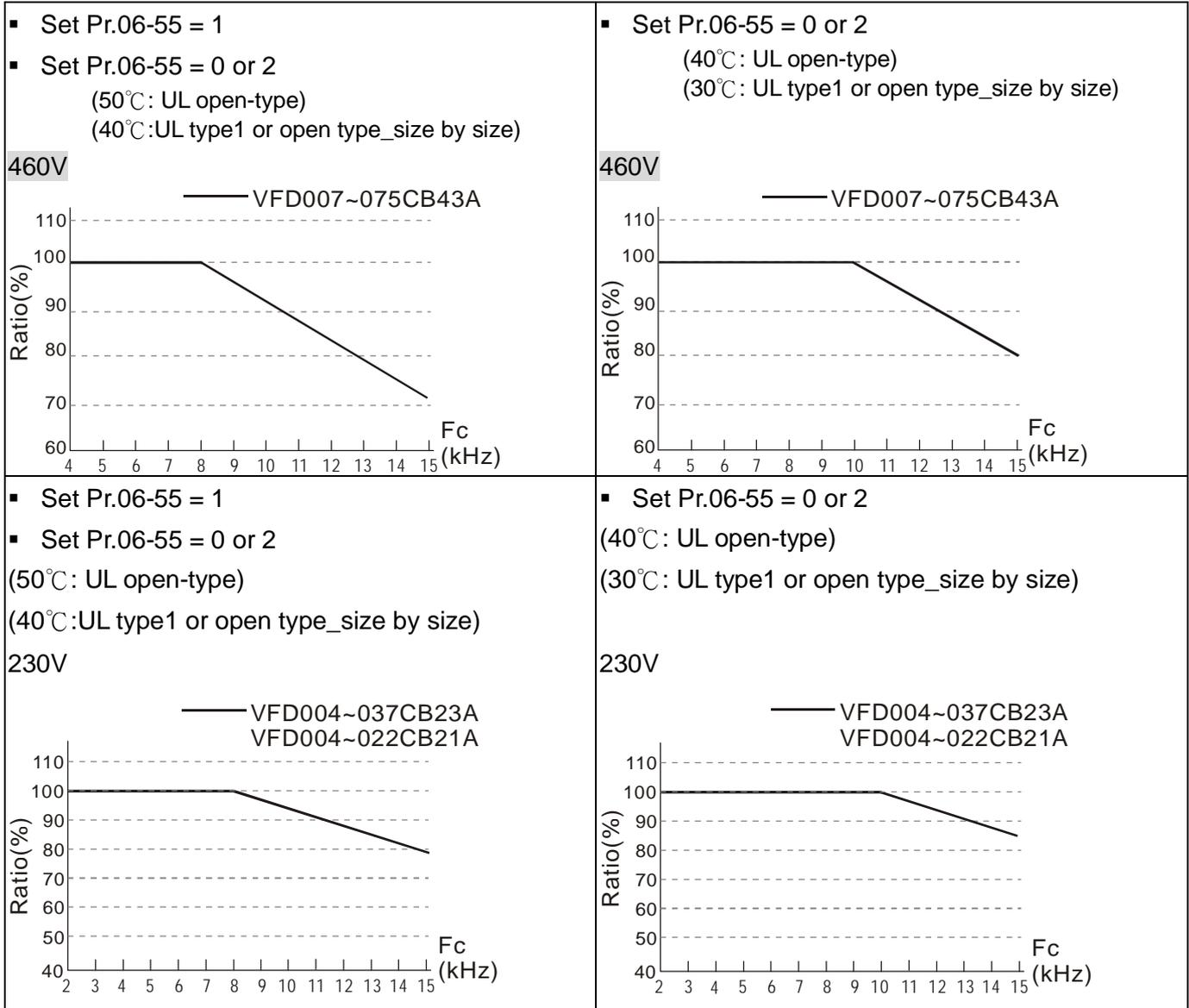
Derating Curve Diagram of Heavy Duty (Pr.00-16=1)
