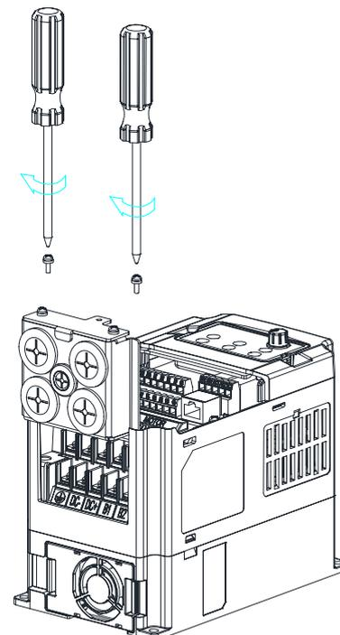
3. Put back the cover then fasten tightly the screw. Screw torque (M3): 6-8Kg-cm(5.2-6.9lb-in.)
