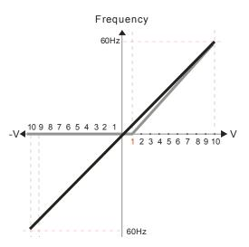
Pr.00-21=0 (Digital keypad control and run in FWD direction) Pr.03-05 Analog Positive Voltage Input Bias (AUI) = 10%
