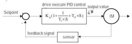
$K_p$ : Proportional gain(P)  $T_i$ : Integral time(I)  $T_d$ : Derivative control(D) S: Operator
