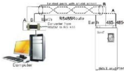
Figure 1 RS485 physical connection in single application
