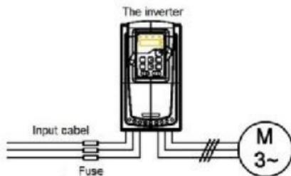
Fig 3-10 Fuse configuration
