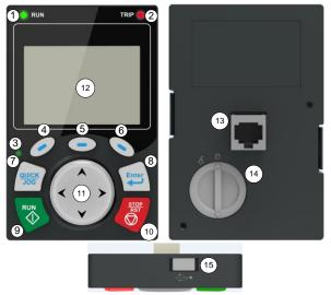
Figure 5.1 Keypad diagram
