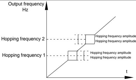
Fig.5-14Skip frequency schematic diagram
