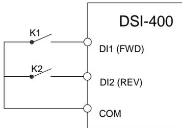
Fig. 5-7 Two-line control mode 2
