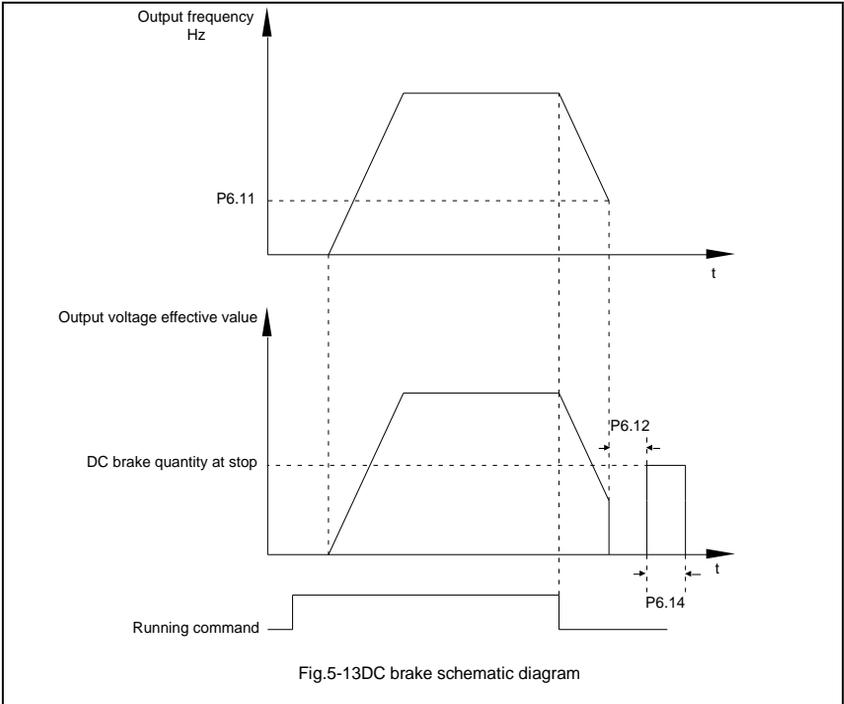
Fig.5-13DC brake schematic diagram
