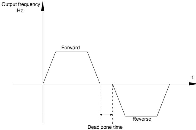
Fig.5-15Rotation dead zone time schematic diagram
