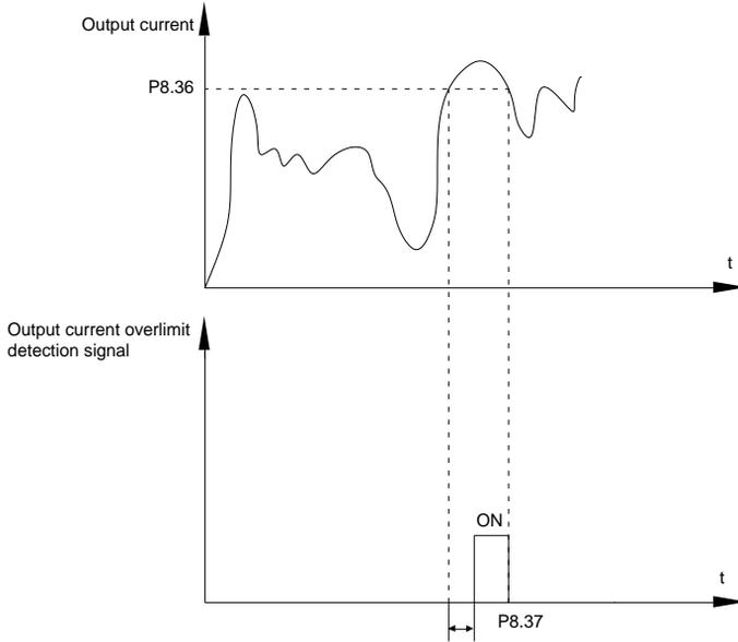
Fig.5-22 Output current over limit detection schematic diagram
