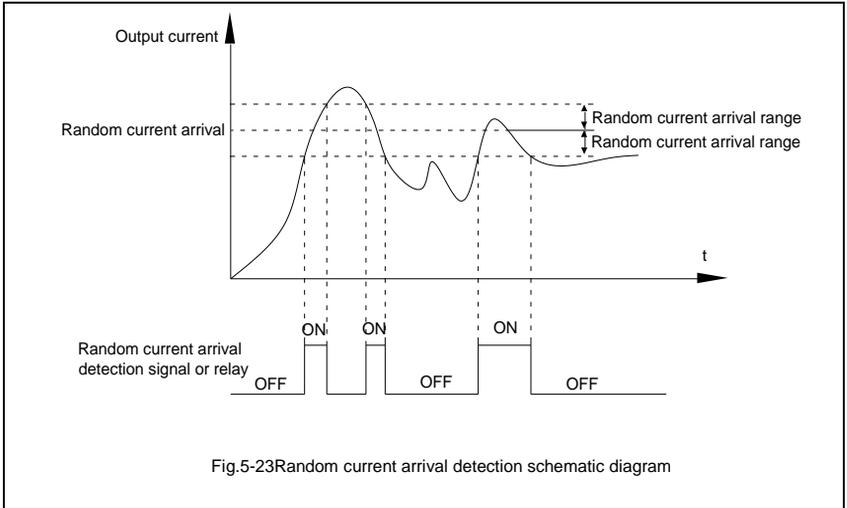
Fig.5-23 Random current arrival detection schematic diagram
