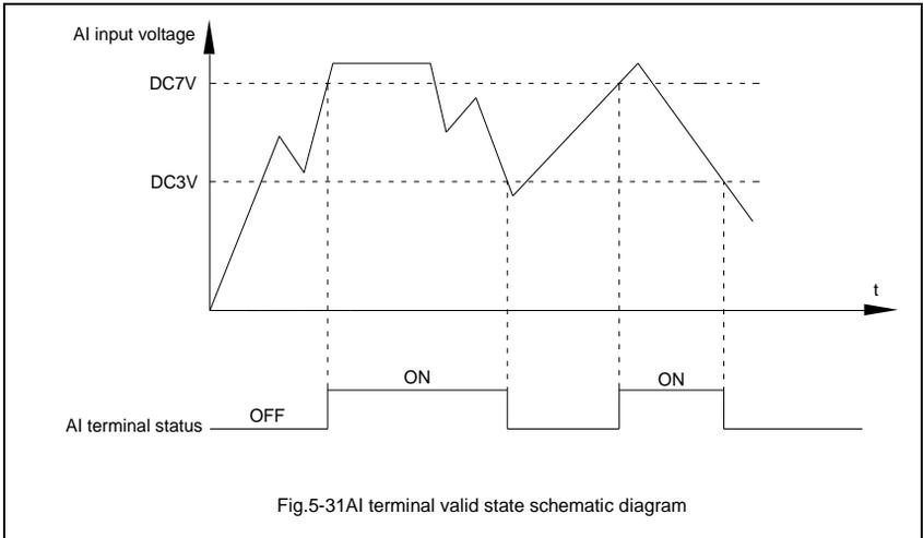
Fig.5-31AI terminal valid state schematic diagram
