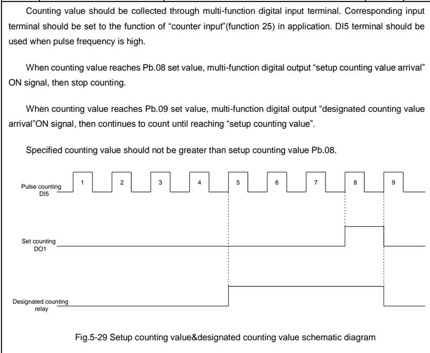
Fig.5-29 Setup counting value&designated counting value schematic diagram
