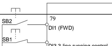
Fig. 5-9 Three-line control mode 2
