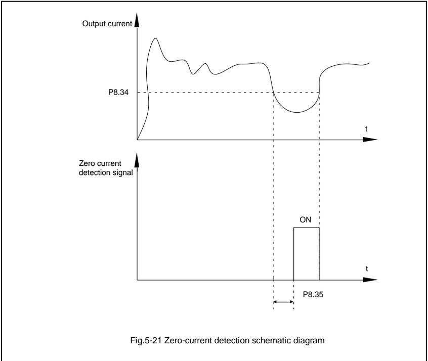
Fig.5-21 Zero-current detection schematic diagram
