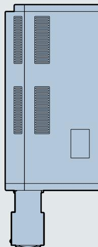
**Note:** Mounting NEMA 1 conduit option to the 15~90kW (20~125HP) Open Type meets NEMA 1 but does not comply with UL Enclosed Type 1. To that end, please purchase UL Type 1 product.
