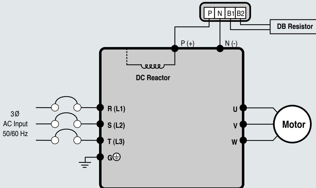
For 37~90kW (50~125HP) Built-in DCL Type
