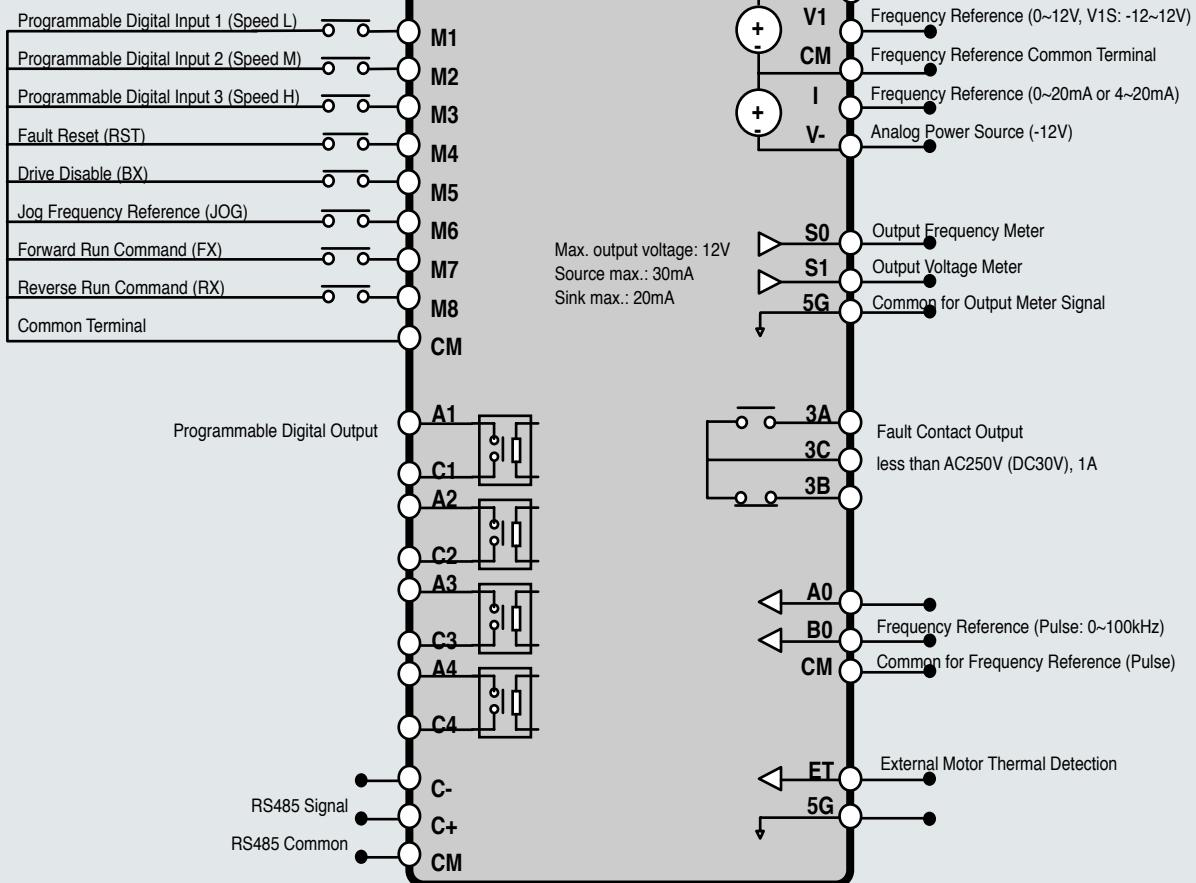
Note 1) 5G is Common Ground for Analog Meter Output (SO, S1) and External motor thermal detection (ET).
