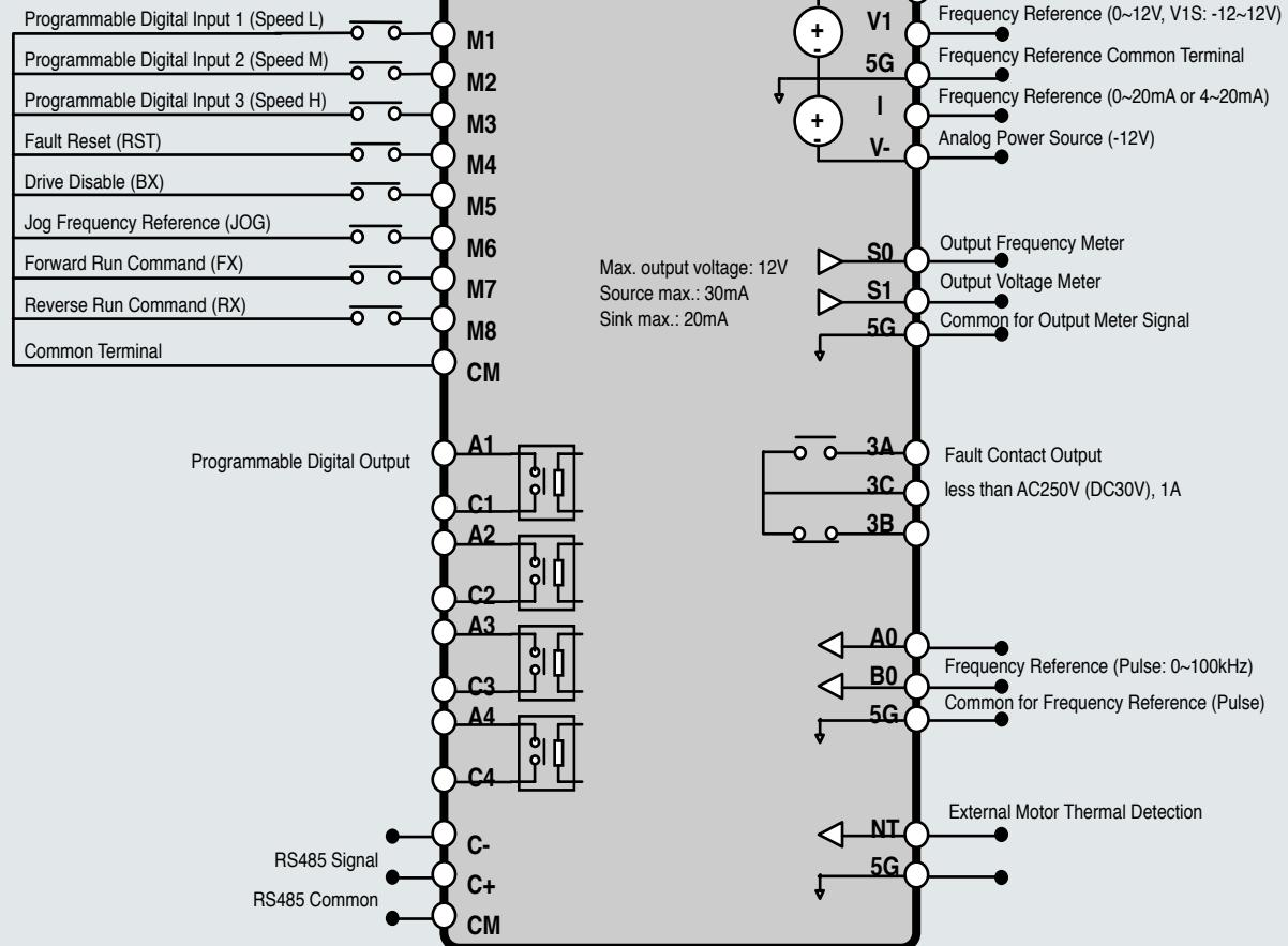
Note 1) 5G is Common Ground for Analog Input / Output.
