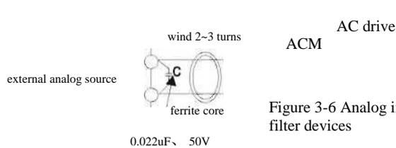
Figure 3-6 Analog input terminal with filter devices
