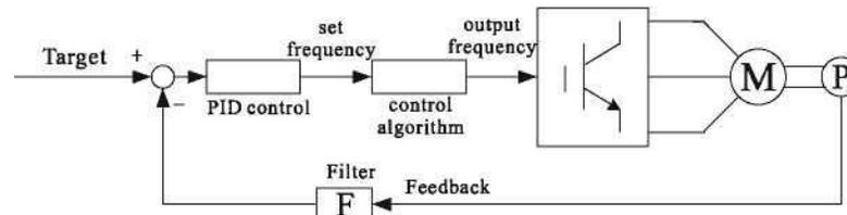
Figure 6-28 Principle block diagram of PID control
