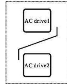
Explanation: When AC drive is installed upside and underside, please install thermal insulation guide plate as picture shows.
