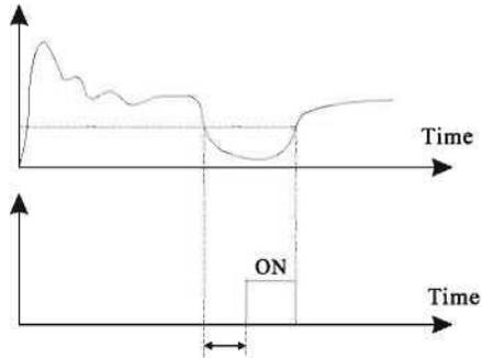
Figure 6-22 Zero current detection
