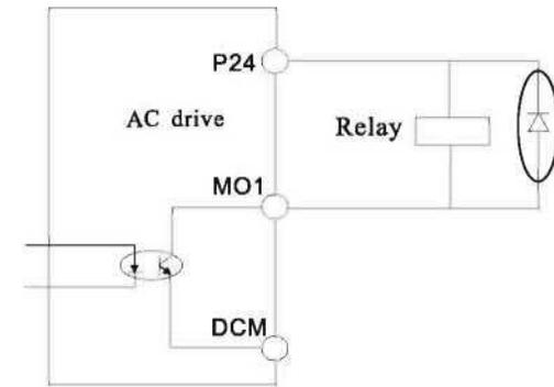
Figure 3-7 Wiring diagram of digital output terminal
