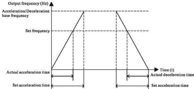
Figure 6-1 Acceleration/Deceleration time
