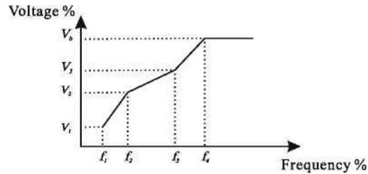
V1-V3: 1 st, 2nd and 3rd voltage percentages of multi -point V/F      F1-F3: 1 st, 2nd and 3rd frequency percentages of multi -point V/F
