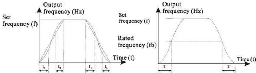
Figure 6-2 S-curve acceleration/deceleration A Figure 6-3 S-curve acceleration/deceleration B
