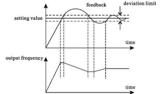
Figure 6-29 relation between deviation limit and output frequency
