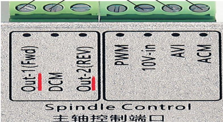
Spindle connected stepper or servo drives
