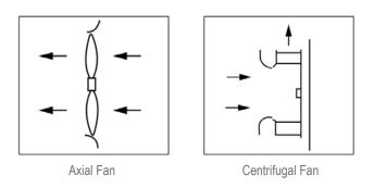
Considering the high static pressure and the outlet shape, these type of fans could be connected to the ductwork. Therefore, due to its ability to overcome the high pressures, centrifugal fans are mostly used at projects with ductworks or other ordinary ventilation equipment like filters.
