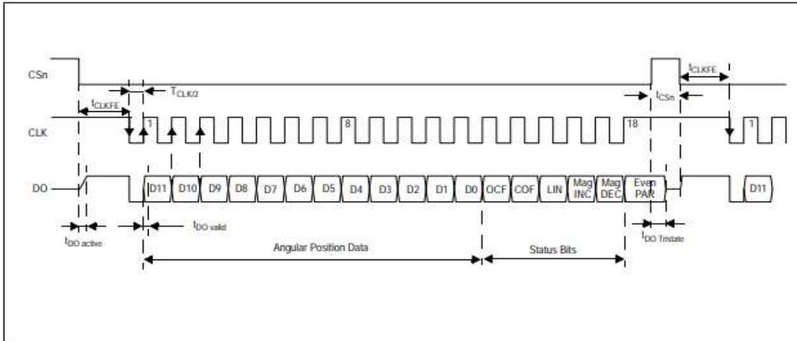
If CSn changes to logic low, Data Out (DO) will change from high impedance (tri-state) to logic high and the read-out will be initiated.
