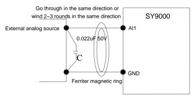
Fig.2-6.2 Analog input terminal processing wiring diagram
