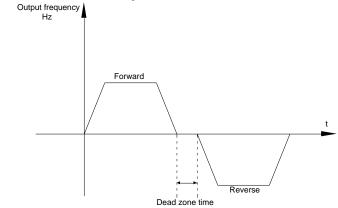
Fig.5-15Rotation dead zone timeschematicdiagram
