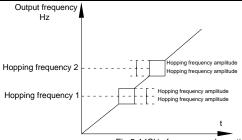
Fig.5-14Skip frequency schematicdiagram
