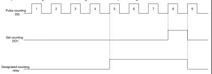
Fig.5-28 Setup counting value&designated counting value schematic diagram
