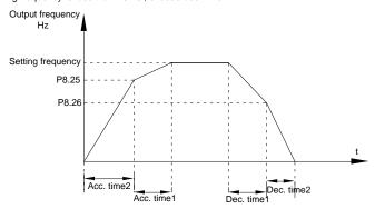
Fig.5-19 Acc./dec. timeswitching schematic diagram
