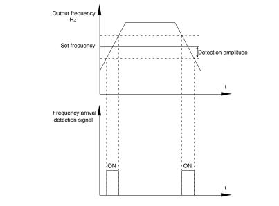
Fig.5-17 Frequency arrival detection amplitude schematic diagram
