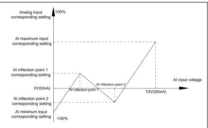
Fig.5-31 Curve4 and curve 5 schematic diagram
