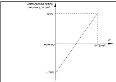
Fig. 5-10 Relationship between analog input and setup value
