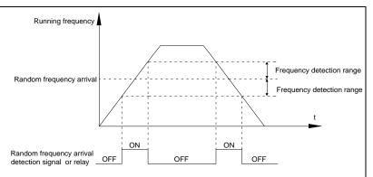
Fig.5-20 Ffrequency arrival detection schematic diagram
