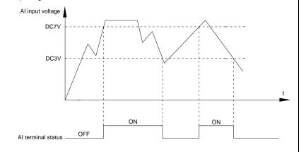
Fig.5-30 Al terminal valid state schematic diagram
