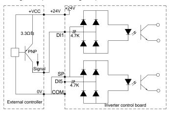
Fig. 2-6.4 Source wiring mode
