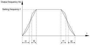
Fig.5-11S-curve acceleration/deceleration schematicdiagram A
