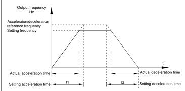
Fig.5-1Acceleration/decelerationtime schematic diagram
