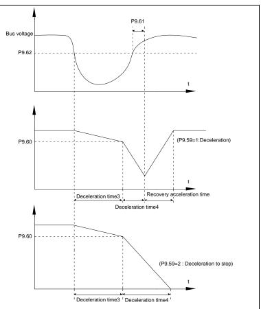
Fig.5-24 Transient stop action schematic diagram
