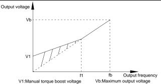
f1:Cutt-off frequency of torque boost fb:Rated running frequency
