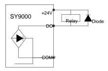
Fig. 2-6.5 Digtal output terminal wiring diagram
