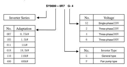
GP unification Model description Users check factory models through P0.00. P type is one lower power than G type.
