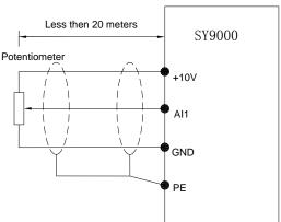
Fig. 2-6.1 Analog input terminal wiring diagram
