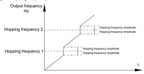
Fig.5-18 Acc./dec. hopping frequency validity schematic diagram
