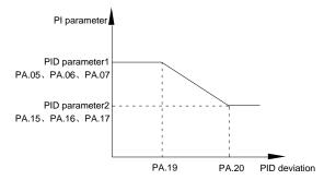
Fig.5-26 PID parameter switching schematic diagram
