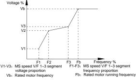
Fig. 5-4 Multi-point V/F curve setup schematic diagram
