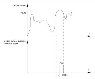
Fig.5-22 Output current overlimit detection schematic diagram
