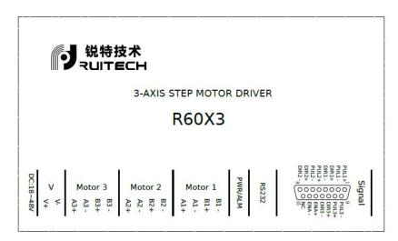
The current and subdivision parameters are set by the R60X3 special debugging software. The driver has over-voltage, under-voltage, and over-current protection. The input and output control signals are optically isolated.
