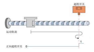
(2) The forward limit switch signal is valid when the motor starts to move The motor directly reverses the forward limit switch signal to the -P290 setting point, and immediately stops after encountering the downward edge of the forward limit switch signal, then searchs for the forward limit switch signal ascent slings at the P290 setting point, and in the process of positive acceleration or forward uniform operation, the forward limit switch signal is immediately stopped.
