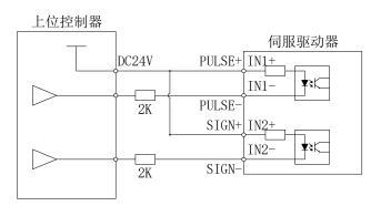
3. Using a single-terminating method, an external common input signal, such as a positive/reverse signal:
