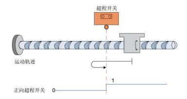
Origin Zero: Forward zero, deceleration point, origin is positive limit switch(P288 x4)
