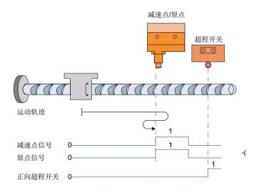
2 The origin switch (deceleration point) signal is valid when the motor is running and no forward limit switch is triggered
