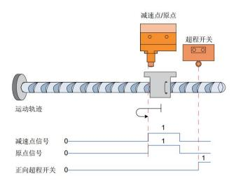
The origin switch (deceleration point) signal is invalid when the motor is starting to run and the forward limit switch is triggered in the process
