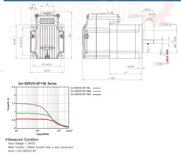
\* : There are 2 kinds size of front shaft diameter for Ezi-SERVO-BT-56 series as  $\Phi$ 6,35 and  $\Phi$ 8,0,
