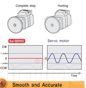
Ezi-SERVO<sup>®</sup> is a high-precision servo drive, using a high-resolution encoder with 32,000 pulses/revolution.
